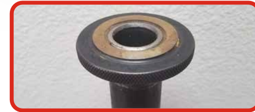
Threads on a new connector passing the thread inspection
