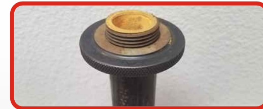
Threads of a worn connector failing the thread inspection
